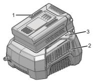
This is a diagnostic charger. The Charger LED Light (3) illuminates in a specified order to show the current battery status. They are as follows:
